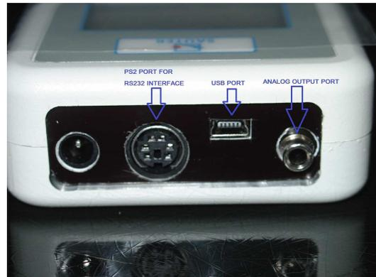
RS-232 and USB: 8 data bits, 1 Start bit, 1 Stop bit, no parity
